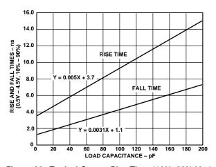
Figure 29. Typical Output Rise Time (10%–90%  $V_{\rm DD}$ ) vs. Load Capacitance ( $V_{\rm DD}$  = 5 V)
