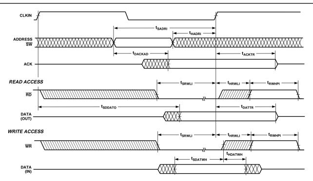
Figure 16. Synchronous Read/Write—Bus Slave
