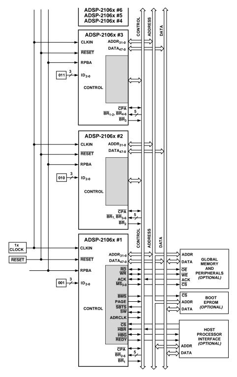
Figure 3. Shared Memory Multiprocessing System
