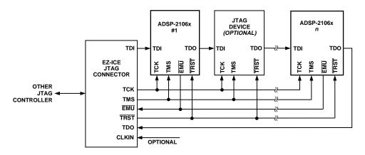
Figure 6. JTAG Scan Path Connections for Multiple ADSP-2106x Systems
