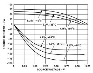
Figure 28. ADSP-21062 Typical Drive Currents ( $V_{DD} = 5 V$ )
