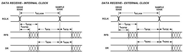
NOTE: EITHER THE RISING EDGE OR FALLING EDGE OF RCLK, TCLK CAN BE USED AS THE ACTIVE SAMPLING EDGE.
