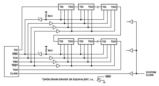
Figure 7. JTAG Clocktree for Multiple ADSP-2106x Systems
