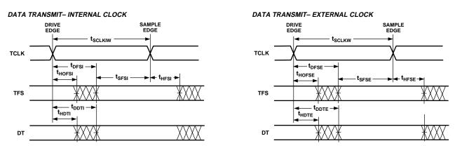
NOTE: EITHER THE RISING EDGE OR FALLING EDGE OF RCLK, TCLK CAN BE USED AS THE ACTIVE SAMPLING EDGE.
