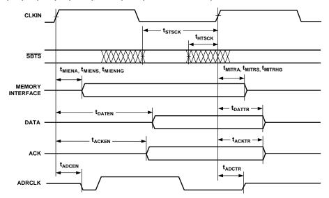
Figure 19a. Three-State Timing (Bus Transition Cycle, SBTS Assertion)
