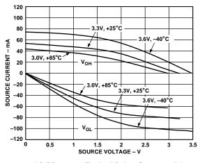
Figure 32. ADSP-21062 Typical Drive Currents ( $V_{DD} = 3.3 V$ )
