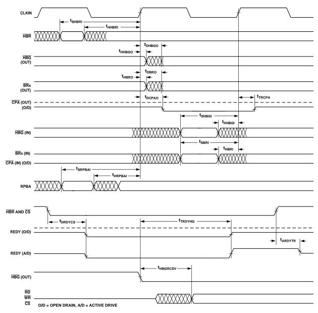
Figure 17. Multiprocessor Bus Request and Host Bus Request
