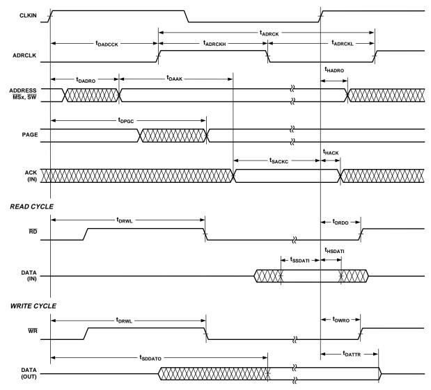
Figure 15. Synchronous Read/Write—Bus Master
