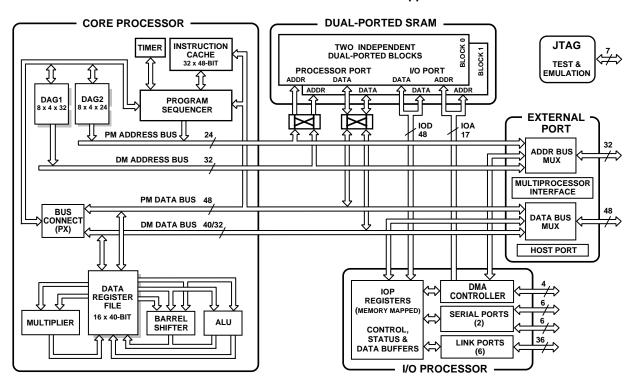
Figure 1. ADSP-21062/ADSP-21062L Block Diagram
