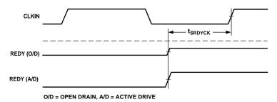
Figure 18a. Synchronous REDY Timing
