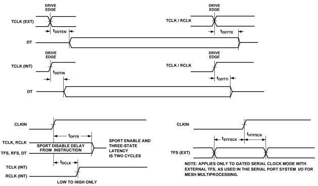
Figure 22. Serial Ports
