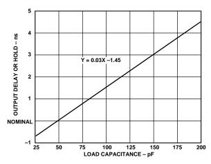
Figure 31. Typical Output Delay or Hold vs. Load Capacitance (at Maximum Case Temperature)  $(V_{DD} = 5 V)$
