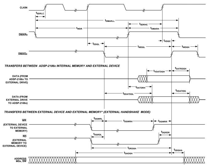
\*MEMORY READ – BUS MASTER, MEMORY WRITE – BUS MASTER, AND SYNCHRONOUS READ/WRITE – BUS MASTER TIMING SPECIFICATIONS FOR ADDR $_{31-0}$ ,  $\overline{\text{ND}}$ ,  $\overline{\text{WR}}$ ,  $\overline{\text{SW}}$ ,  $\overline{\text{MS}}_{3-0}$  AND ACK ALSO APPLY HERE.
