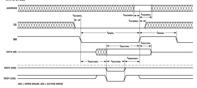
Figure 18b. Asynchronous Read/Write—Host to ADSP-21062
