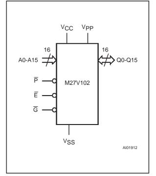
Figure 2A. DIP Pin Connections
