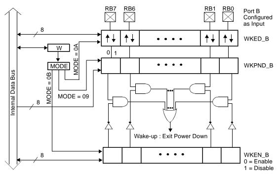
Figure 7-1. Multi-Input Wakeup Block Diagram
