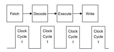
Figure 15-1. Pipeline and Clock Scheme
