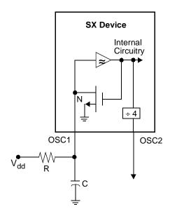
Figure 9-3. RC Oscillator Mode
