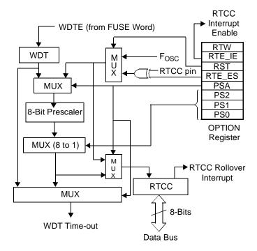
Figure 10-1. RTCC and WDT Block Diagram
