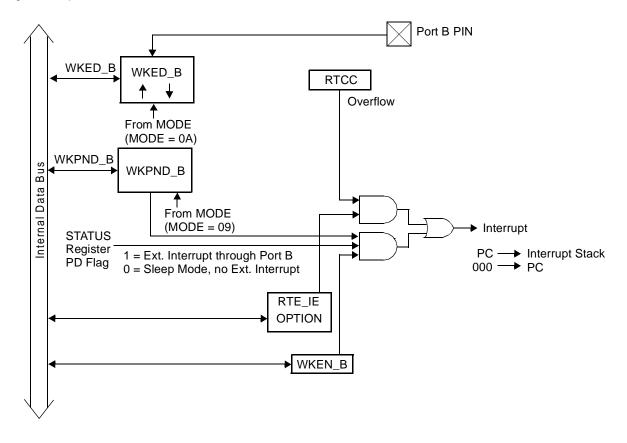
Figure 8-1. Interrupt Structure
