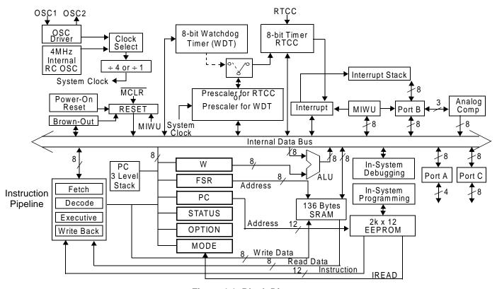
Figure 1-1. Block Diagram
