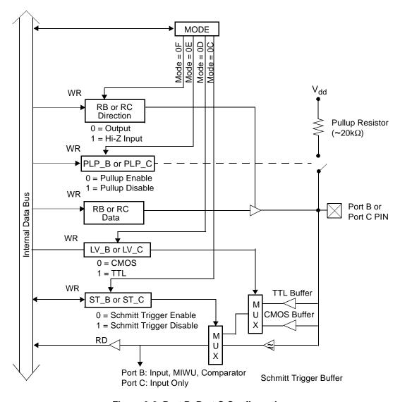
Figure 3-2. Port B, Port C Configuration
