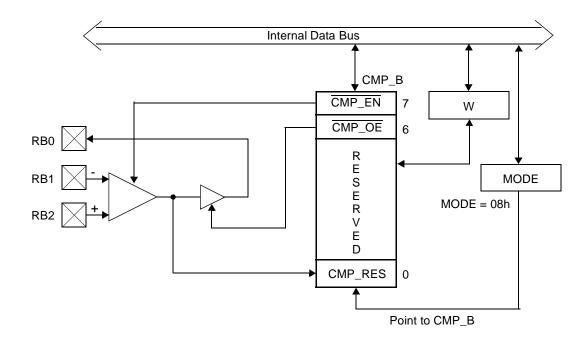
Figure 11-1. Comparator Block Diagram
