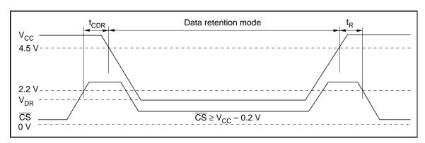
Low  $V_{CC}$  Data Retention Timing Waveform ( $\overline{CS}$  Controlled)
