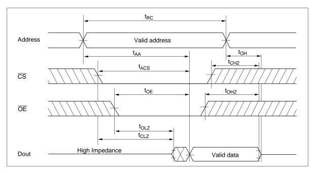
Read Timing Waveform (2)  $(\overline{WE}=V_{IH},\,\overline{CS}=V_{IL},\,\overline{OE}=V_{IL})$
