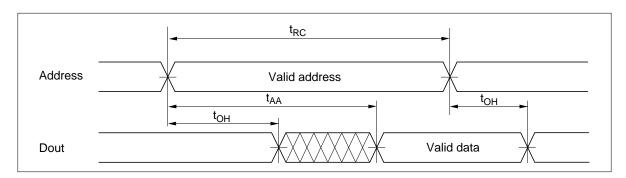
Read Timing Waveform (3)  $(\overline{WE}=V_{IH},\overline{CS}=V_{IL},\overline{OE}=V_{IL})^{*2}$
