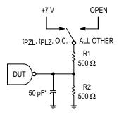
\*includes all probe and jig capacitance
