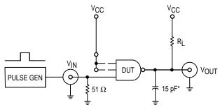
\*includes all probe and jig capacitance
