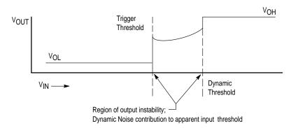
The V<sub>IN</sub> versus V<sub>OUT</sub> plot shows the practical effect of testing noise on a logic IC device. The actual device *Trigger threshold* is represented by the initial low to high output transition. The device will oscillate if the input voltage does not exceed the trigger threshold plus the noise generated by the interaction of the test system or given application with the device.
