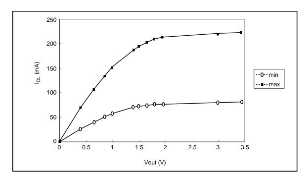
Output High Current (I $_{OH}$ ) (Ta = 0 to 65°C, V $_{CC}$  = 3.0 V to 3.45 V, V $_{SS}$  = 0 V)
