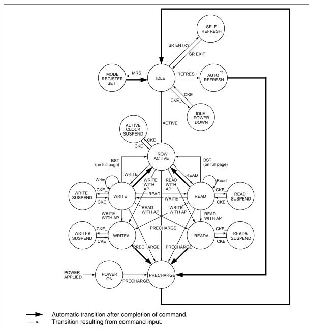
Note: 1. After the auto-refresh operation, precharge operation is performed automatically and enter the IDLE state.
