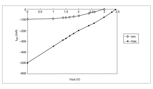
**DC Characteristics** (Ta = 0 to +70°C,  $V_{CC}$ ,  $V_{CC}Q = 3.3 \text{ V} \pm 0.3 \text{ V}$ ,  $V_{SS}$ ,  $V_{SS}Q = 0 \text{ V}$ ) (HM5212165F)
