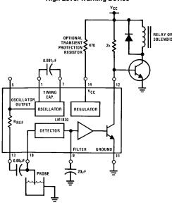
The Output is suitable for driving a sump pump or opening a drain valve, etc.
