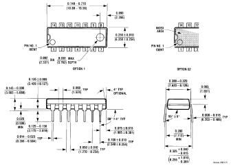
Molded Dual-In-Line Package (N) Order Number LM1830N NS Package Number N14A
