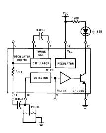
FIGURE 3. Basic Low Level Warning Device with LED Indication
