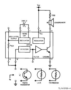
Output is activated when R<sub>p</sub> is approximately greater than 1/3 R<sub>REF</sub> FIGURE 4. Direct Coupled Applications
