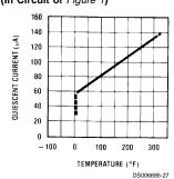
Quiescent Current vs. Temperature (In Circuit of Figure 2; -V<sub>S</sub> = -5V, R1 = 100k)
