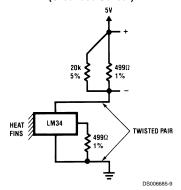
$V_{OUT} = 10 \text{mV/}^{\circ} \text{F} (T_{A} + 3^{\circ} \text{F})$ FROM +3°F TO + 100°F
