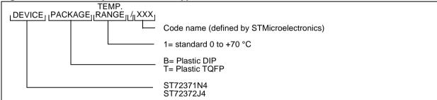
Figure 46. OTP User Programmable Device Types
