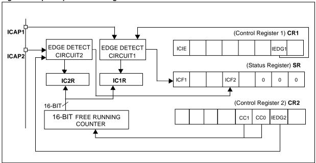
Figure 22. Input Capture Timing Diagram
