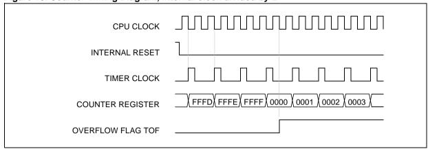
Figure 19. Counter Timing Diagram, internal clock divided by 4
