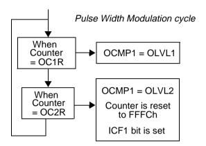
**Note:** After a write instruction to the OC*i*HR register, the output compare function is inhibited until the OC*i*LR register is also written.
