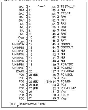
Figure 3. ST72371J 42-Pin SDIP Pinout
