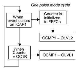
Then, on a valid event on the ICAP1 pin, the counter is initialized to FFFCh and OLVL2 bit is loaded on the OCMP1 pin. When the value of the counter is equal to the value of the contents of the OC1R register, the OLVL1 bit is output on the OCMP1 pin, (See Figure 25).
