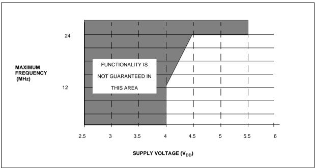
**Note:** The shaded area is outside the recommended operating range; device functionality is not guaranteed under these conditions.
