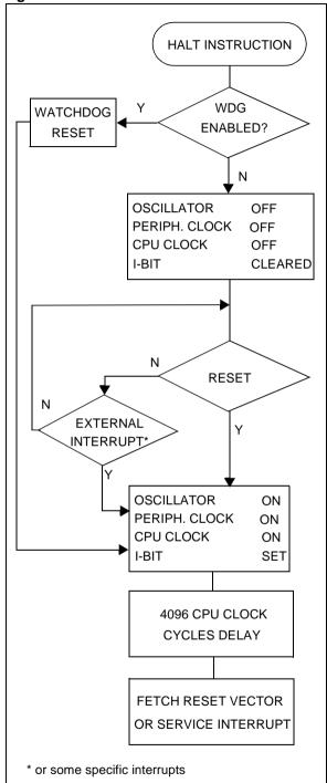
**Note:** Before servicing an interrupt, the CC register is pushed on the stack. The I-Bit is set during the interrupt routine and cleared when the CC register is popped.
