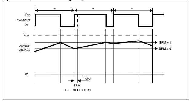
Figure 36. Graphical Representation of 4-Bit BRM Added Pulse Positions
