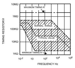
Figure 5. R versus Oscillation Frequency.
