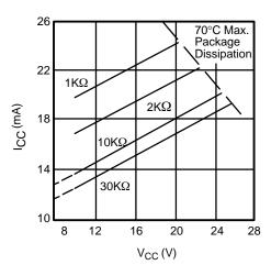
Figure 4. Supply Current vs Supply Voltage, Timing, R.
