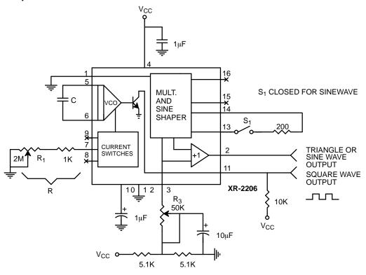
Figure 11. Circuit tor Sine Wave Generation without External Adjustment. (See *Figure 3*. for Choice of R<sub>3</sub>)
