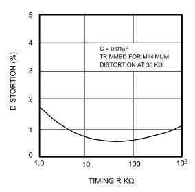
Figure 7. Trimmed Distortion versus Timing Resistor.
