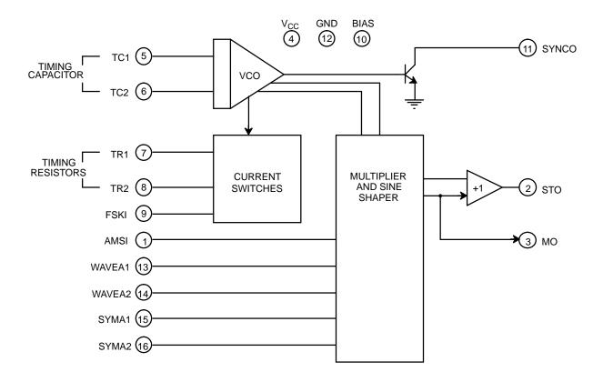
Figure 1. XR-2206 Block Diagram.
