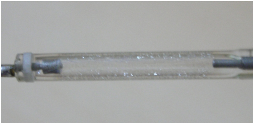
Fig. 3. Interior damaged Xenon tube due to intense light burst caused by a high energy discharge.
