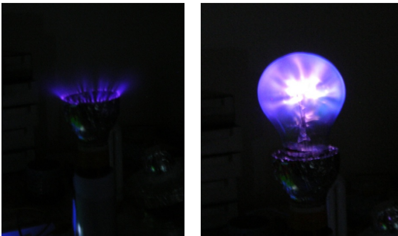
Fig. 2. Streamers emanating from the secondary terminal. A light bulb is acting as a plasma globe.
