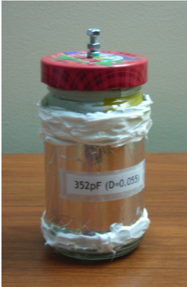
Fig. 3. A simple jar capacitor, easy to manufacture and cheap. The lower value of the capacitance has some advantages. First, since the HV supply charges the capacitor rapidly, the spark-gap firing rate is very high compared to a larger capacitor version. Second, since the accumulated charge is low, the risk of electrical shock is also low.
